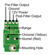
Figure 1: Int. Module Connections
